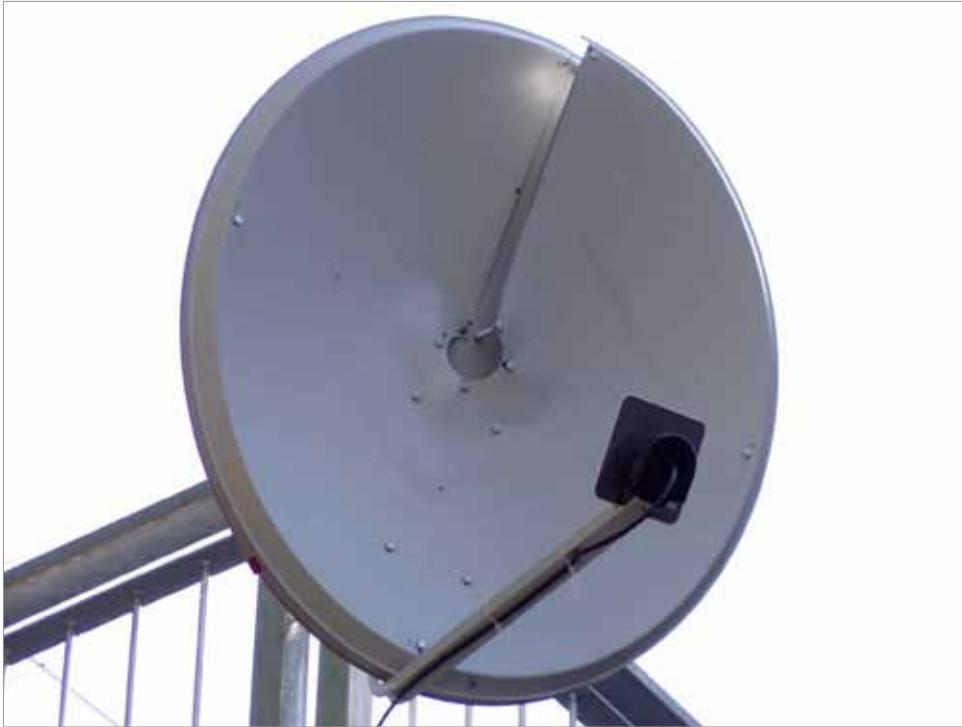
**SLIGHT TWIST:** Bending a dish antenna let researchers project twisted radio waves.
